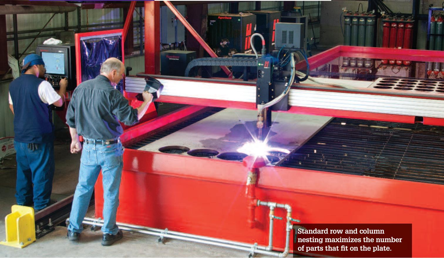
Standard row and column nesting maximizes the number of parts that fit on the plate.
